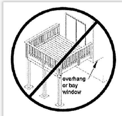
**NOTE:** YOU MAY NOT ATTACH LEDGER BOARDS TO EXISTING CANTILEVERS, OPEN WEB TRUSSES OR STONE OR MASONRY VENEER. If these conditions occur, the deck must be freestanding. If a freestanding deck is utilized, then it must be braced diagonally to resist lateral loads.
